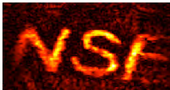
Figure 1. (Left) Resistive heating effects for the prototype MR-stage microscope gradient set. Airflow insulating/cooling effect. Adding airflow reduces the temperature rise on the surface of RF coil to less than 1.0 C. (Right) High speed MR microscopy. Gradient echo EPI acquired using the prototype MR-stage microscope. The image represents a 500 \mu\text{m} slice through a plastic phantom with hollow character spaces filled with 1mM Prohance solution. Nominal in-plane resolution is 100 \mu\text{m} x 100 \mu\text{m} with a total imaging time of 26 ms.
